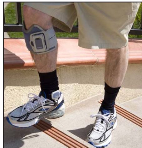
The NESS L300 is an advanced foot drop system designed to use mild stimulation to lift the foot to help patients walk more safely and easily.
